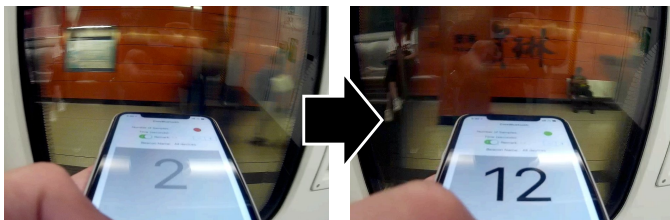
Fig. 4: Video screenshot of experiments with fast speed inside metro station. The number of received packets is indicated.
